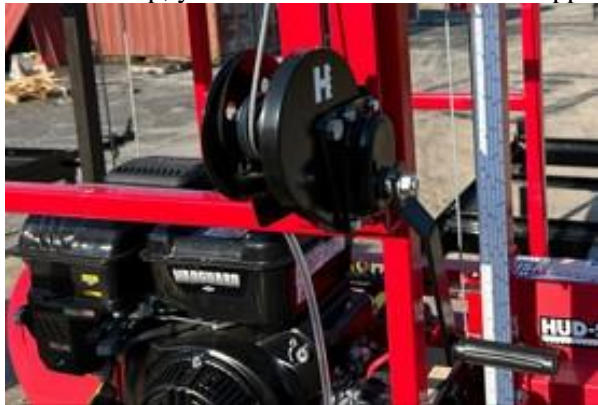
Correct head placement: Operators side is on side with the scale stick And hand winch.
