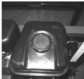
Gasoline fuel tank
