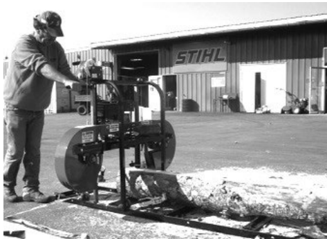
#3. Adjust blade height, rev engine.
