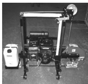
Lift tubes: keep Clean and oil lightly daily.
