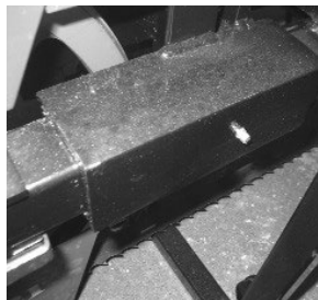
Tensioner slide, (grease weekly)
