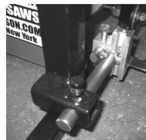
Guide assembly, keep clean and lightly oil all parts.
