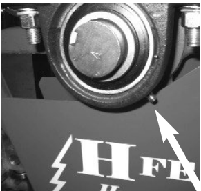
Grease all bearings weekly or as needed.
