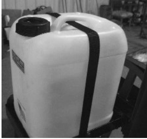
Lube tank for blade lube.
